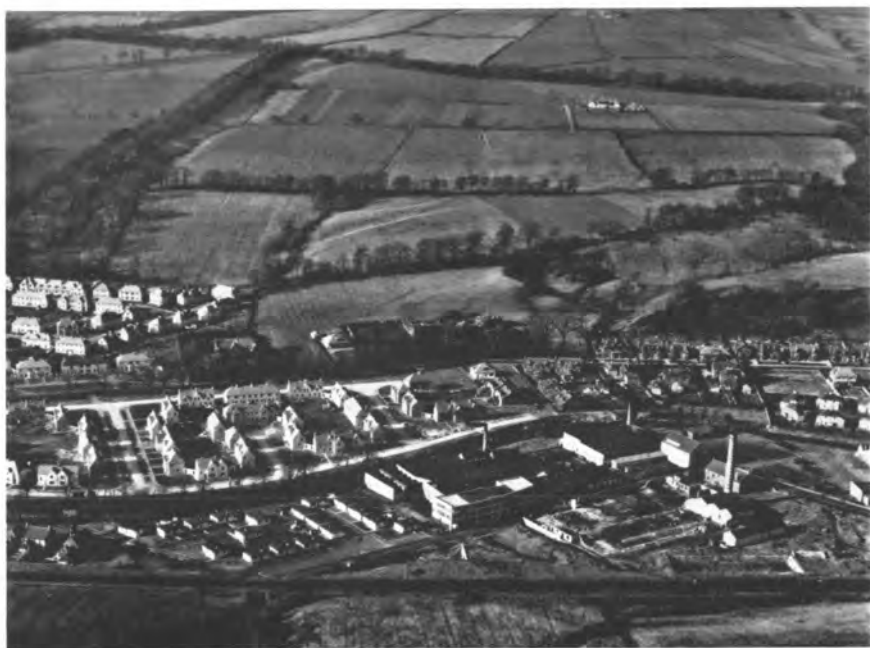
Plate 10. The Darvel valley, Newmilns, Ayrshire, looking north across the town and mills built on alluvial land (map unit 1) to undulating lowland of map unit 331 in the Kilmarnock Association. The thick tills which underlie this land are typical of central Ayrshire. The soils are slowly permeable. SDD Crown Copyright
